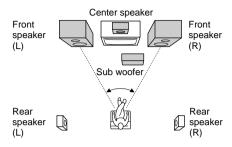
2 Place the center speaker at about the same height as the front speakers. Align the center speaker with the front speakers or place it slightly behind the front speakers.
